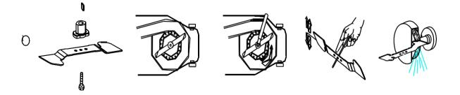
To remove the blade, loosen the screw, check the blade bracket, and replace all parts if they are worn or damaged.
