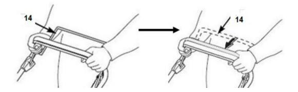
To stop the mower, release the self-propelled lever and then the brake lever.
